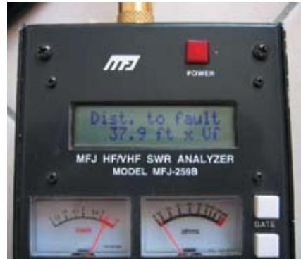
Slika 4. Distance to fault izražen u Ft
